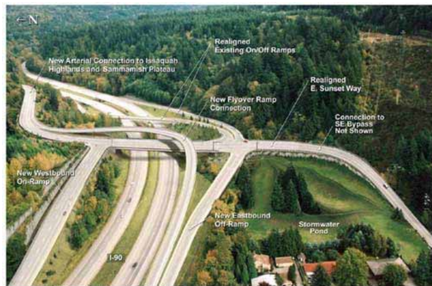
Conceptual Alternative 1 View of the Project Area South SPAR and Sunset Interchange Modification
