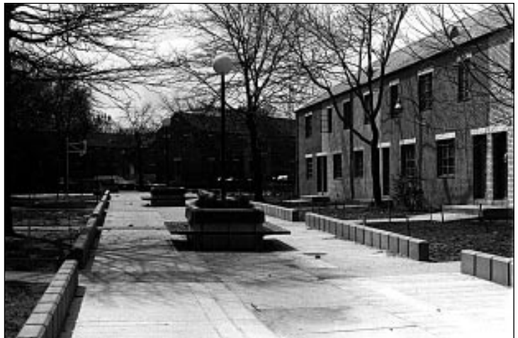
Figure III-5: Collective front yards are defined by the new concrete curbing. A new combination lighting, seating, and planter helps residents use and identify with the central walk.
