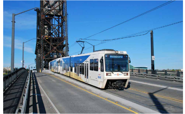
Four light-rail lines meet to have as many as 16 trains per hour cross this bridge, but elsewhere in Portland light rail runs no more than 12 trains per hour. Since Portland light-rail trains can have no more than two cars, that means few lines can carry more than 3,600 people per hour. Photo by Steve Morgan.
