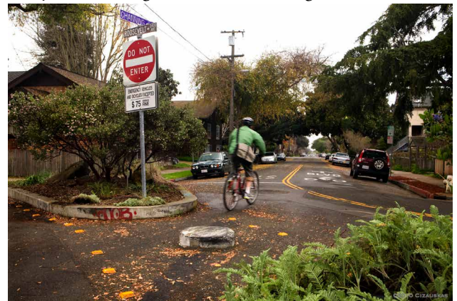
Bicycle boulevards, such as this one in Berkeley, use local streets parallel to major collectors or arterials and apply a few barriers to allow local automobile traffic and through bicycle traffic. Photo by Carrie Cizauskas.
