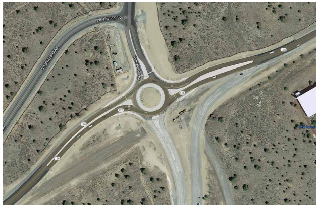
This roundabout forces traffic on the heavily used east-west road to slow from 65 to 25 mph, sometimes causing long back-ups, in order to avoid a traffic light or overpass for the lightly used north-south road. A larger roundabout would have allowed faster speeds and avoided congestion.
