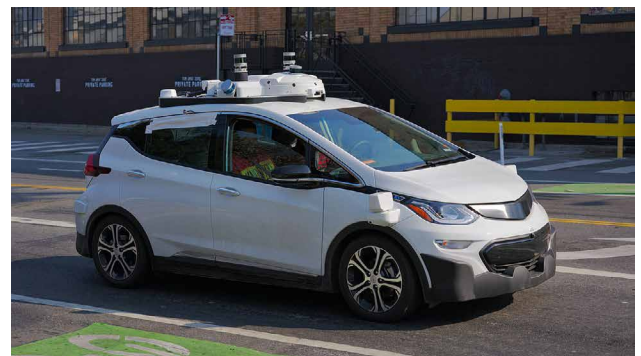
This General Motors' Cruise vehicle is making LIDAR maps of San Francisco. Click here to watch a YouTube video in your browser about how Here is making such maps. Photo by Dllu.
