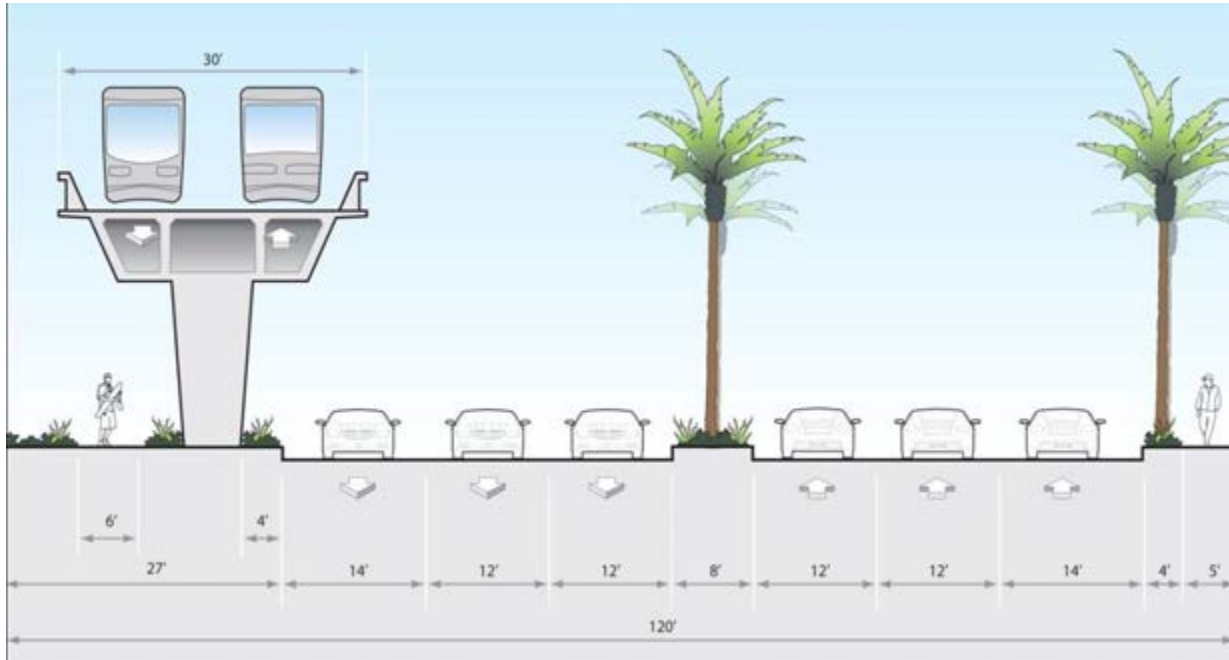
Figure ES.9 – Elevated Fixed-Guideway Alternative: Typical Cross-Sections
